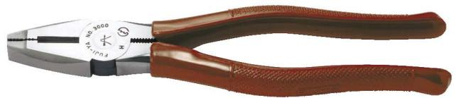
Easy cutting of 3 cored VA cables by specially-milled hexagonal hole at the reverse side of edges. 225mm is equipped with Crimping function from Crimping sizes 1.25-5.5mm.
