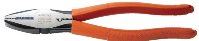
Super higher cutting ability increased by 20% by cutting-edge technology "MICRO MIRROR BALDE" developed by our latest engineering know-how. Easy cutting of 3 cored VA cables by specially-milled hexagonal hole at the reverse side of edges with Crimping function from Crimping sizes 1.25-5.5mm.
